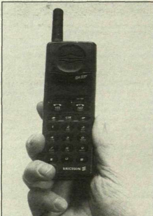
Ericsson's smallest pocket phone for GSM, the GH337, has been a tremendous success in 1994. This phone is also available in versions for most of the other mobile standards. It's weight is only about 200 grammes.
