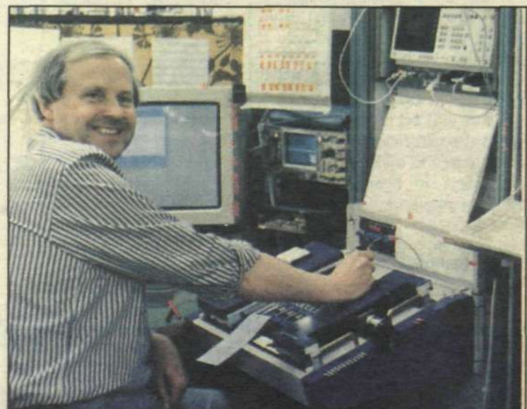
Lennart Gustavsson looks for faults in ALEs (analog line interface boards) in ACA 3. All boards are tested during production and those that prove to be faulty are sent to Lennart.
