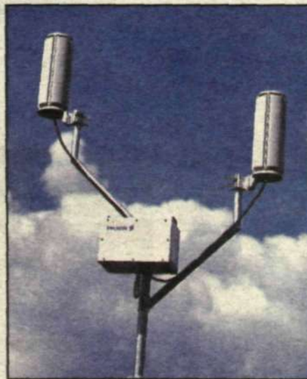
The base station (DECT access node) covers the requirements of up to 600 subscribers and has a range of a few kilometers.
