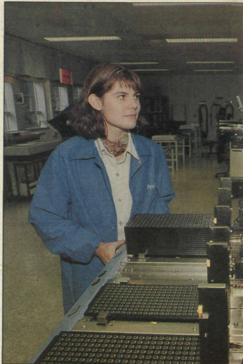
The Pick-and-Place handler (the accepted term in this context) places circuits on a tray and positions them for measurement. The process is wholly automated and can operate several hours unmanned. Susanne Fiebig-Halldén runs radio circuits and ASIC circuits for the business center for ASIC, terminals, power and IC circuits. Photo: Anders Anjou
