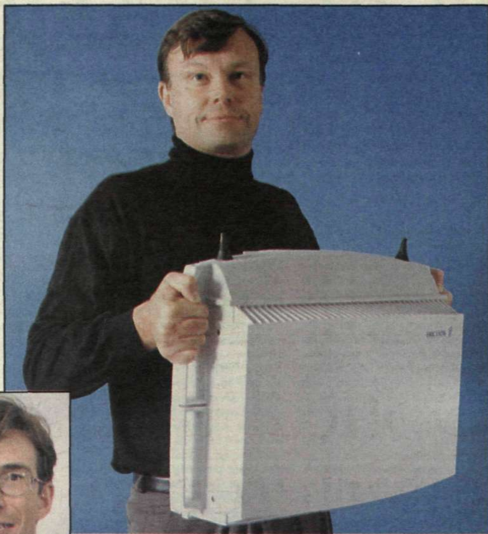
The prototype version of the world's smallest base station for mobile telephony is portable and weighs less than 25 kilograms. (above)
