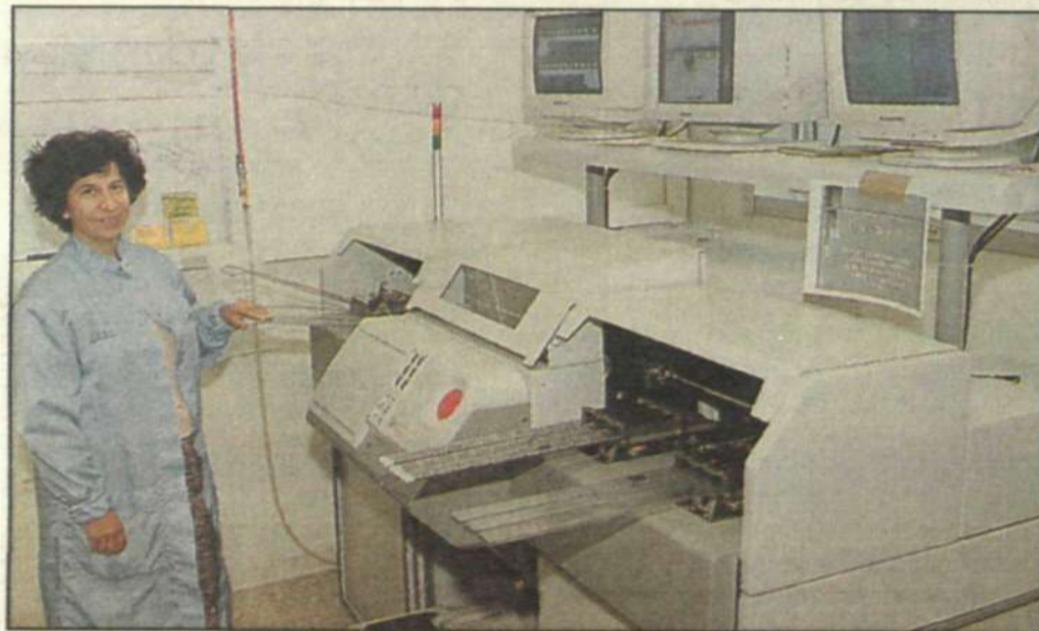
Francisca Abatté scans components to determine if any of the legs were damaged following encapsulation. This visual inspection is preceded by an electrical inspection.
