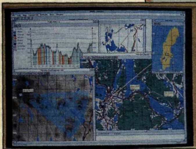
The screen displays the Ludvika area in Sweden, with maps of surrounding areas to facilitate calculations of link paths; terrain profile of the path is shown in the upper left-hand corner. The so-called sight-coverage diagram can be seen in the lower left-hand corner; it is used to identify suitable sites for transmitters. The unmarked sections indicate areas with good coverage.
