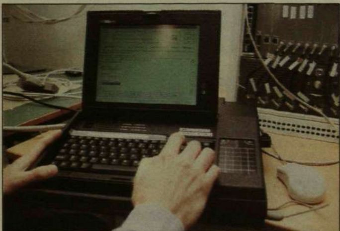
The Stand Alone Test Tool tests hardware in the radio base station to ensure that it will work with the switch, independent of the actual switch. Everything is contained in a laptop computer.
