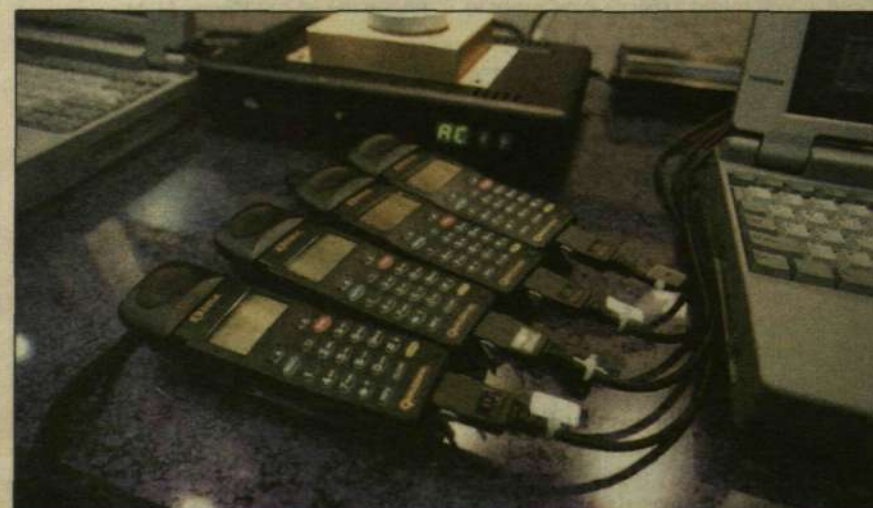
One of Qualcomm's featured attractions at Wireless '97 was a demonstration that showed how CDMA telephones can be used for data communications - without a modem between the telephone and the PC.
