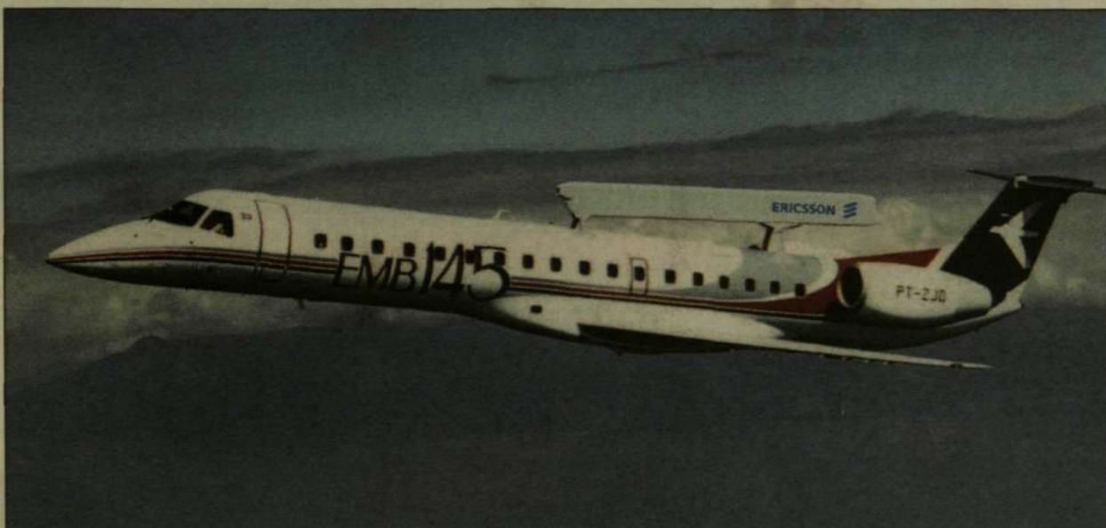
Erieye will be installed on Brazilian 145 Embraer aircraft. The airborne radar surveillance systems from Ericsson will be used in Brazil's Sivam Project to monitor the Amazon rain forests.
