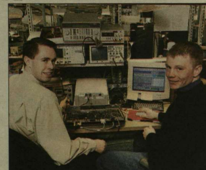
2. When the circuit boards have passed the final mounting stage, including manufacturing of control boards for the microwave unit and baseband boards for the radio unit, it is time for tester Patrik Ramberg to test the parts of the outdoor unit in simulated environment. Here, he is testing a microwave unit, assisted by trainee Mathias Carlsson.
