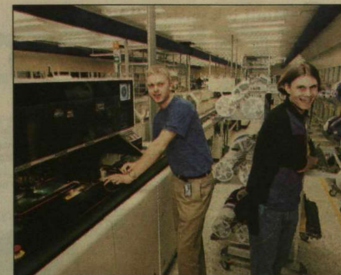
1. The surface mounting of circuit boards is the first step in the manufacturing of a MiniLink. Currently, the Borås plant's two production lines manufacture close to 3,000 circuit boards per week. Operators Joakim Håkansson and Christian Gunnarsson monitor the process, ensuring that mounted components – approximately 25,000 per hour – end up in the right place.
