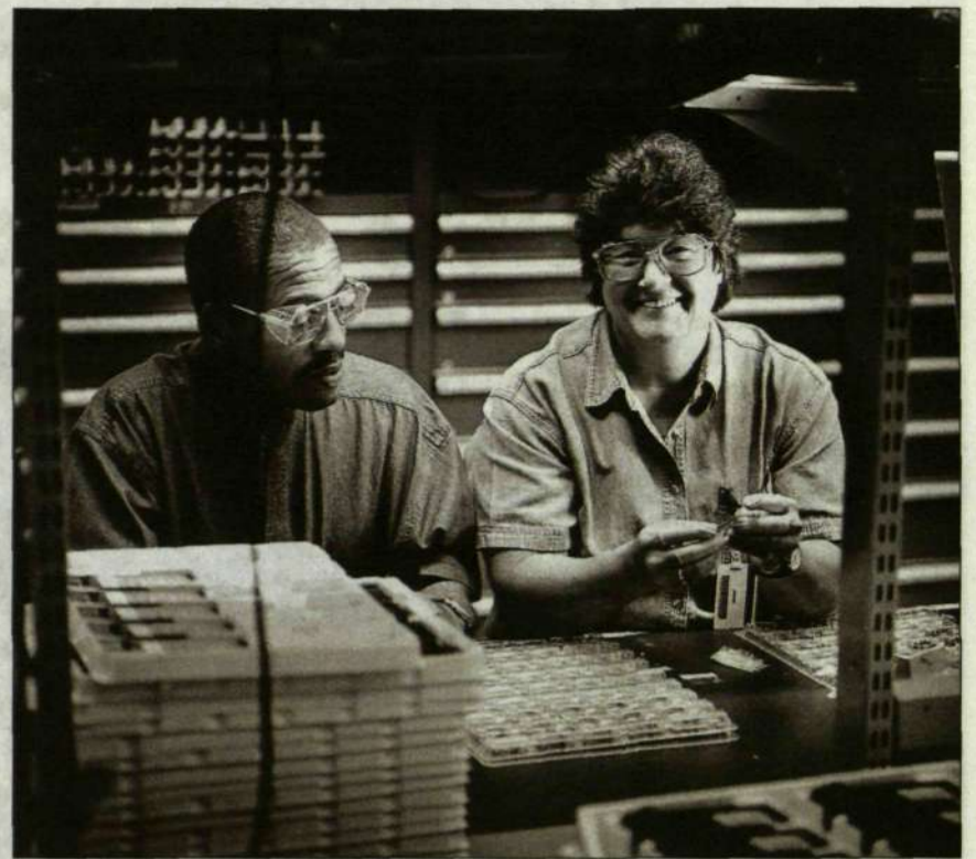
Bud Gaines and Yvonne Gibson look for bubbles in LCD displays of mobile telephones. The bubbles are so small they are difficult to detect with untrained eye. Bud and Yvonne rely on their eyes, however; magnifying glasses are for amateurs.
