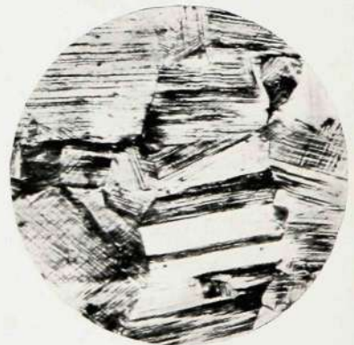
Austenitic Steel Hard Rolled x 200
