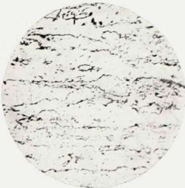
Low Carbon Stainless Iron x 200
