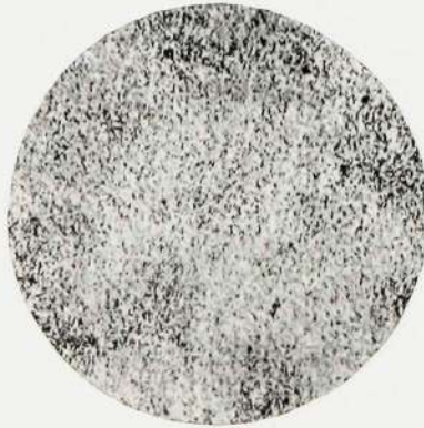
Medium Carbon Stainless Steel x 200
