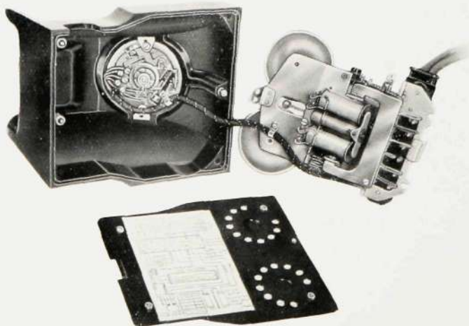
Fig 7—Automatic Table Telephone with apparatus unit removed
