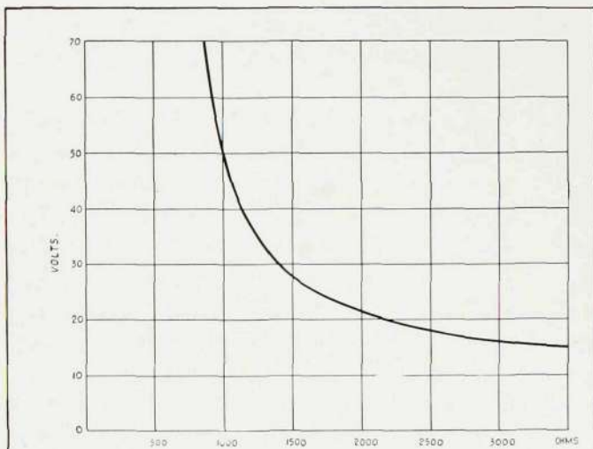
FIG. 1. TYPICAL VOLTAGE RESISTANCE CURVE OF SELECTED "BACK TO BACK" ELEMENTS ASSEMBLY.
