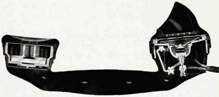
Fig. 9—A Cross-Section of the Bakelite Micro-Telephone
