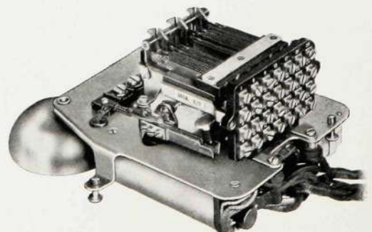
Fig. 10—A Chassis with a 9K Spring-set Key Unit
