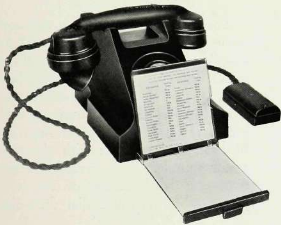
Fig. 4—C.B. Telephone Showing Sliding Tray
