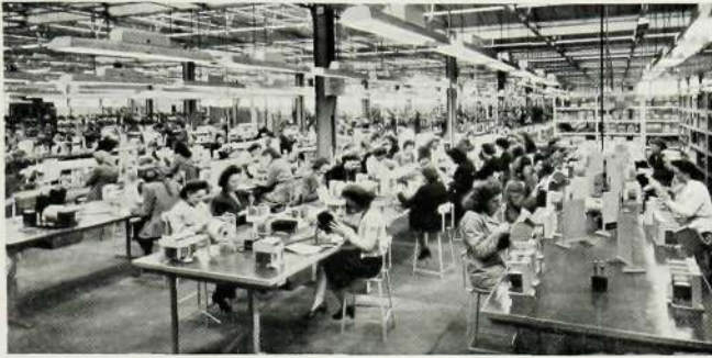
Fig. 4—Wiring Jack-in Relay Sets
