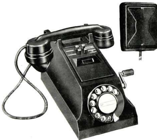
Fig. 1—Intermediate Telephone, External System
