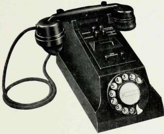
Fig. 3—Intermediate Telephone, Internal System
