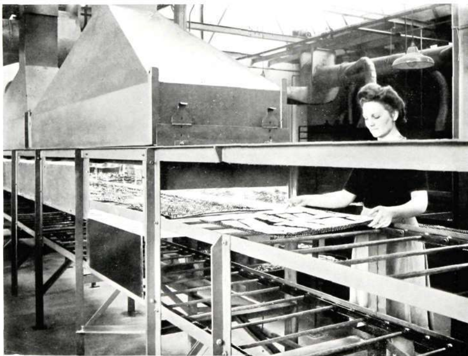
Fig. 3—Parts being fed on to the Conveyor of the Infra-Red Dryer
