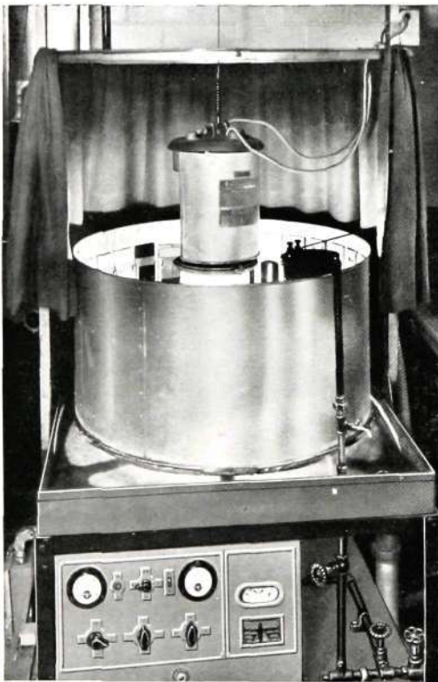
Fig. 1—Accelerated Weathering of Specimen Panels
