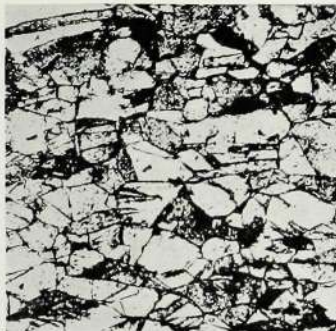
Fig. 22—Cartridge Brass, showing Strain from Extrusion.
