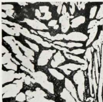
Fig. 10—Isolated Grain Formation in 57 : 43 Brass.
