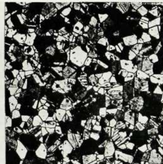
Fig. 23—Cartridge Brass Extruded and Annealed.
