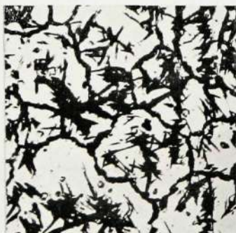
Fig. 17—Cobalt Magnet Steel, Austenitic, Early Transition Stage.
