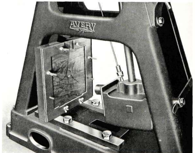
Fig. 3—Wood Laminate Undergoing Impact Test.
