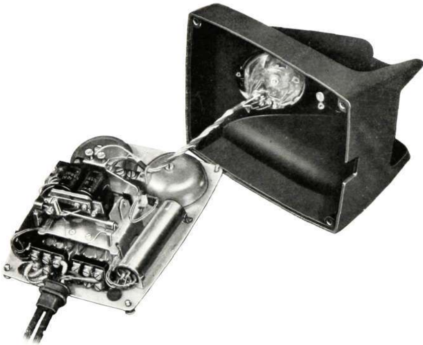
Fig. 4—Extension Set with Case off
