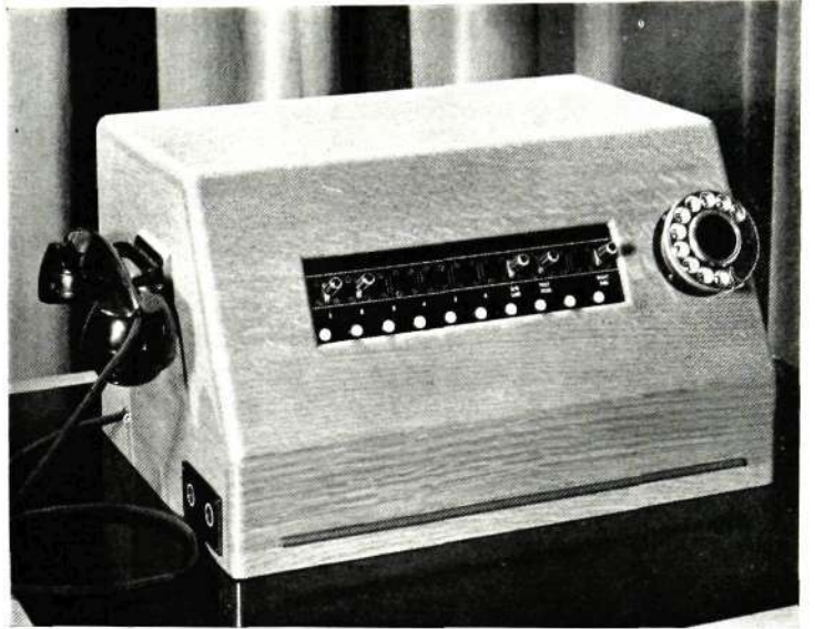
Fig. 8—Repair Service Turret
