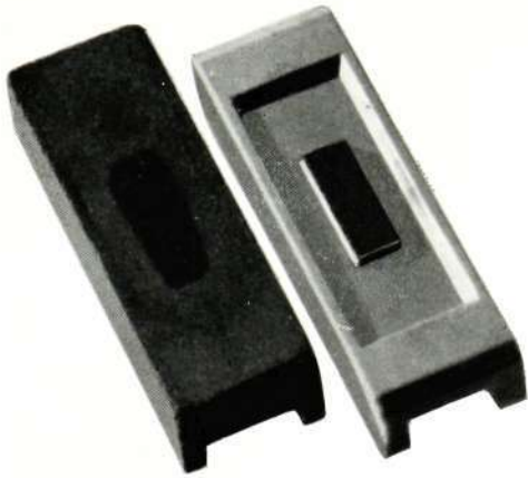
Fig. 6—A Type 236 Protector after subjection to one hundred discharges each of 100 joules at 1500 volts
