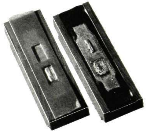
Fig. 9—Showing the effect of one discharge of 100 joules at 1500 volts on a standard British Post Office type Protector
