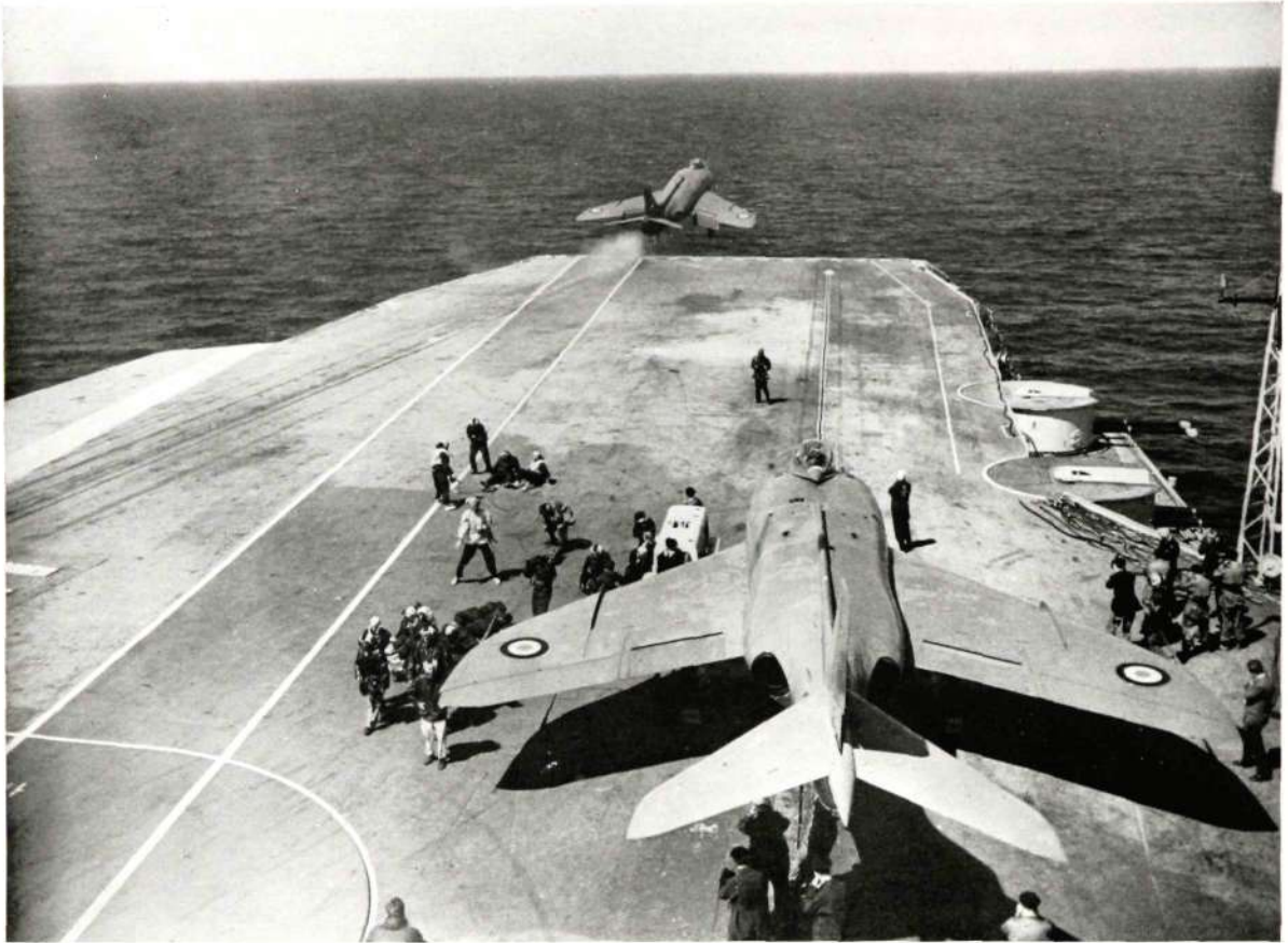
Fig. 1—A Scimitar launched from Ark Royal port steam catapult while another is being prepared for launching from the starboard catapult. (Official Admiralty photograph).
