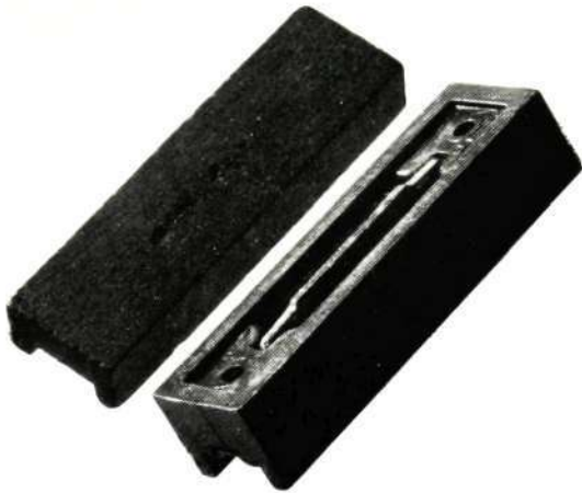
Fig. 8—This 'Knife-edge' Protector, also, shows noticeable damage after one discharge similar to that applied in Fig. 7
