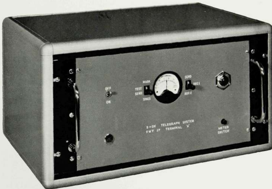
Fig. 6—S + DX Telegraph System FMT. 17 Terminal Equipment
