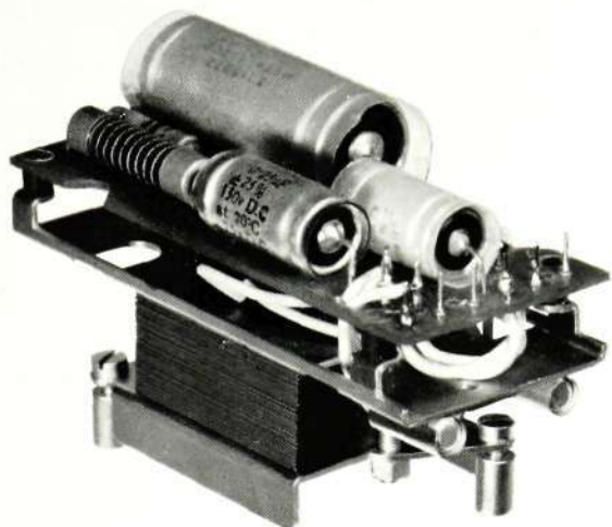
Fig. 3—25 c/s Generator operative from 12 volts d.c. for single-position switchboards
