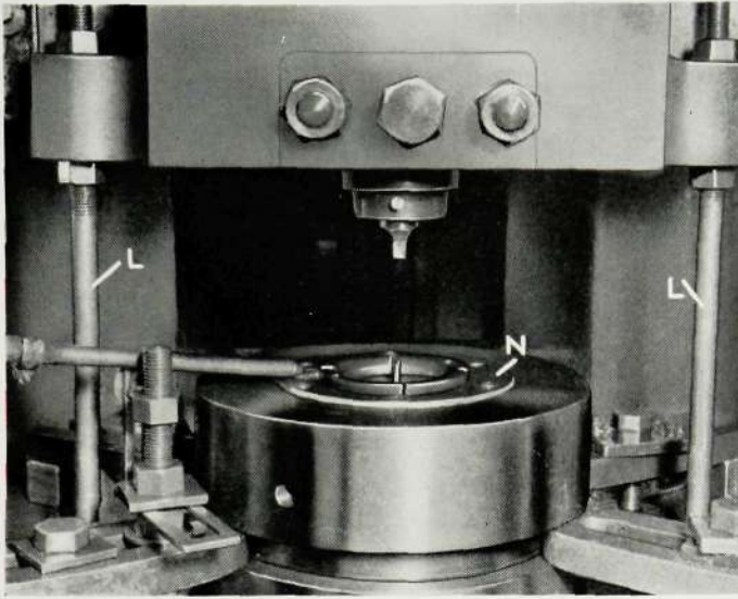
Fig. 3—The fulcrum portions of the yokes are cold headed at the rate of 475 an hour, on a 75-ton press, with the tools here shown
