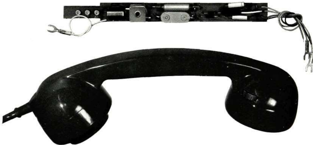
Fig. 1—Complete Handset with Amplifier alongside
