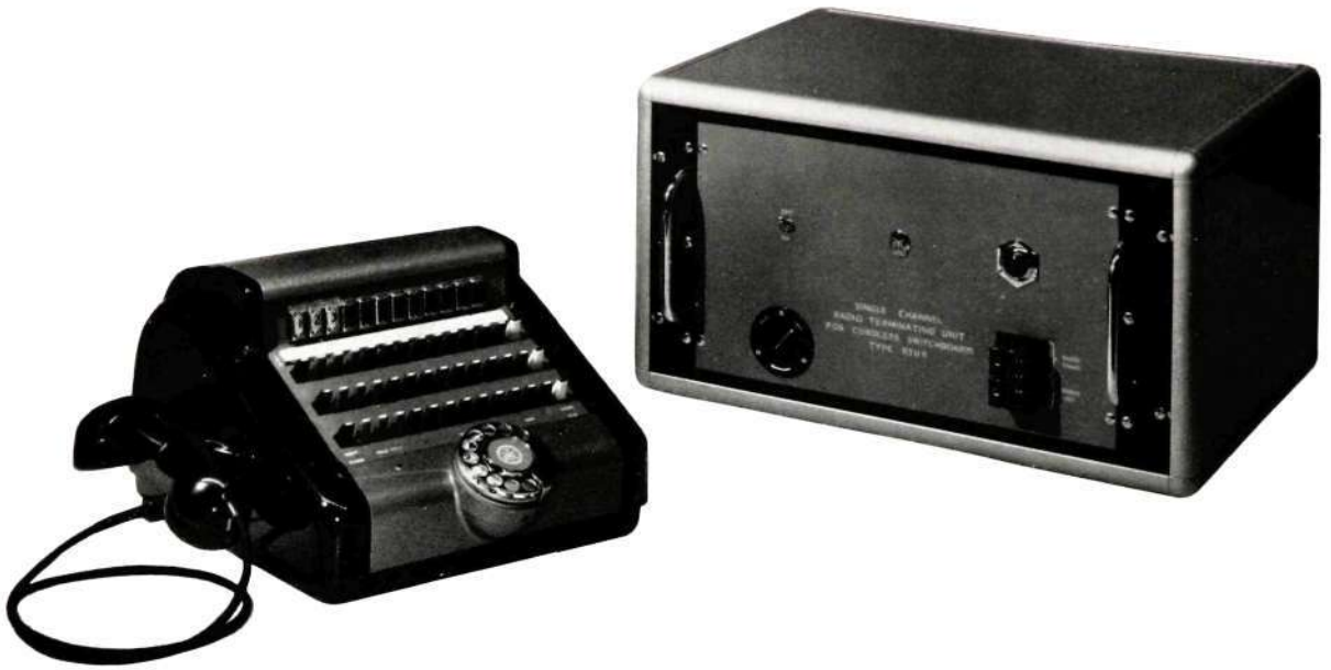
Fig. 4—RTU8 Unit with typical cordless switchboard
