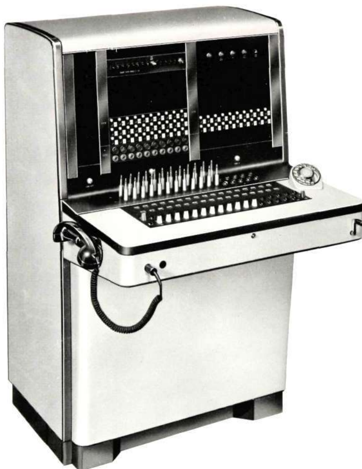
Figure 3—General view of CB Auto Lamp-Signalling Switchboard
