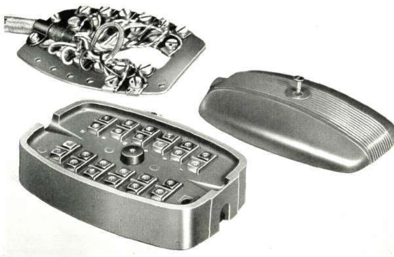
Figure 4 Cord-termination plate before connection to desk-block base
