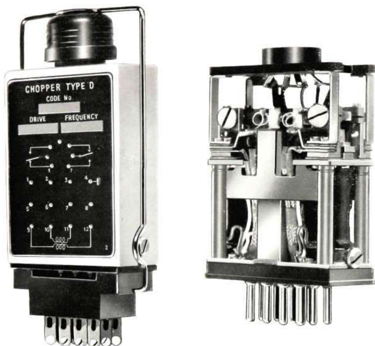
Figure 2—External and internal views of Low-noise Chopper Type 'D'
