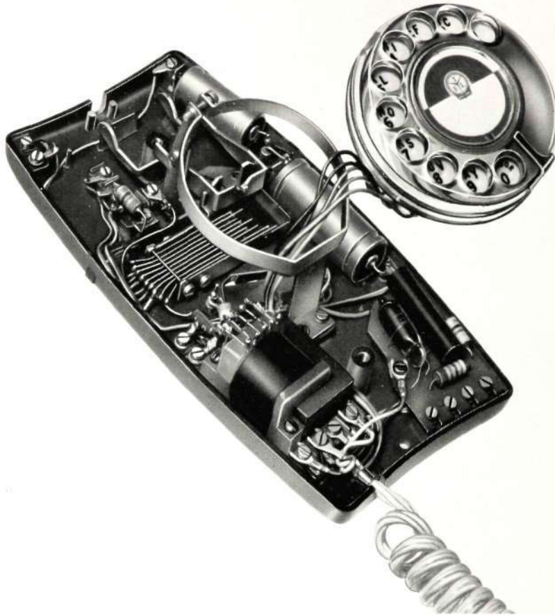
Figure 2—Interior view of the Etelux, with dial removed from its mounting.
