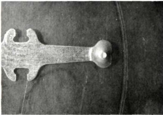
Figure 8—Nickel-silver wiper, s.r.b.p. disc Without lubrication Wiper loss : 40 \mu gms
