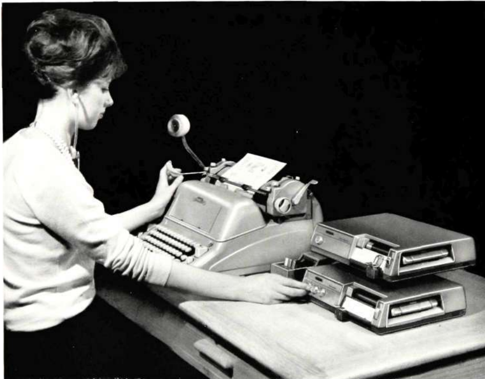
Figure 3—Typical desk layout showing recording machine mounted above transcribing machine
