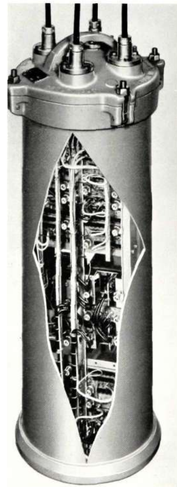
Figure 7—Cut-away photograph showing internal apparatus of intermediate repeater mounted in airtight container for accommodation in concrete manhole
