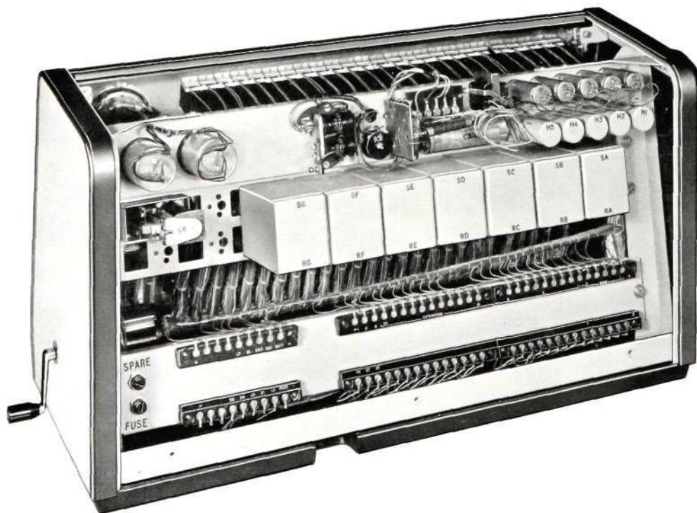
Figure 2—Rear view of switchboard with wrap-over panel removed
