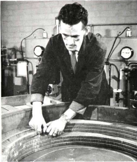
Packing 3000-type yokes for heat treatment after machining. This basket takes 10,000, the cycle lasting 21 hours. Sufficient heat treatment capacity exists for 30,000 complete relay magnetic circuits per day
