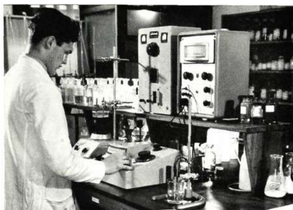
A corner of the laboratory showing calorimetric analysis of factory effluent
