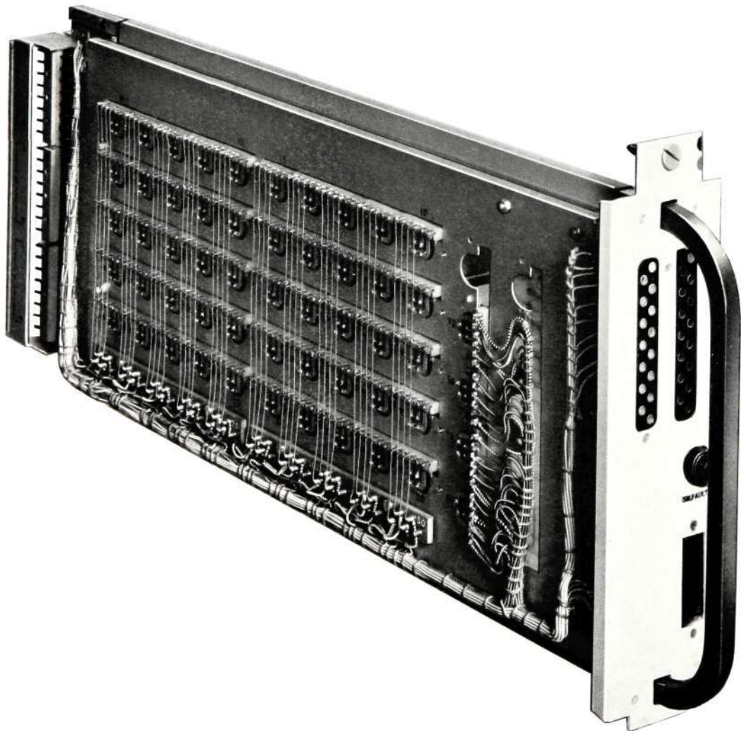
Figure 9—C Switch, showing three access relays TA, TB, TC, and one alarm relay AL, in addition to the 5 × 10 matrix and its vertical wiring multiples
