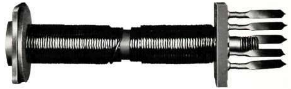
Figure 3—Maranyl A 190 former prepared for winding tests
