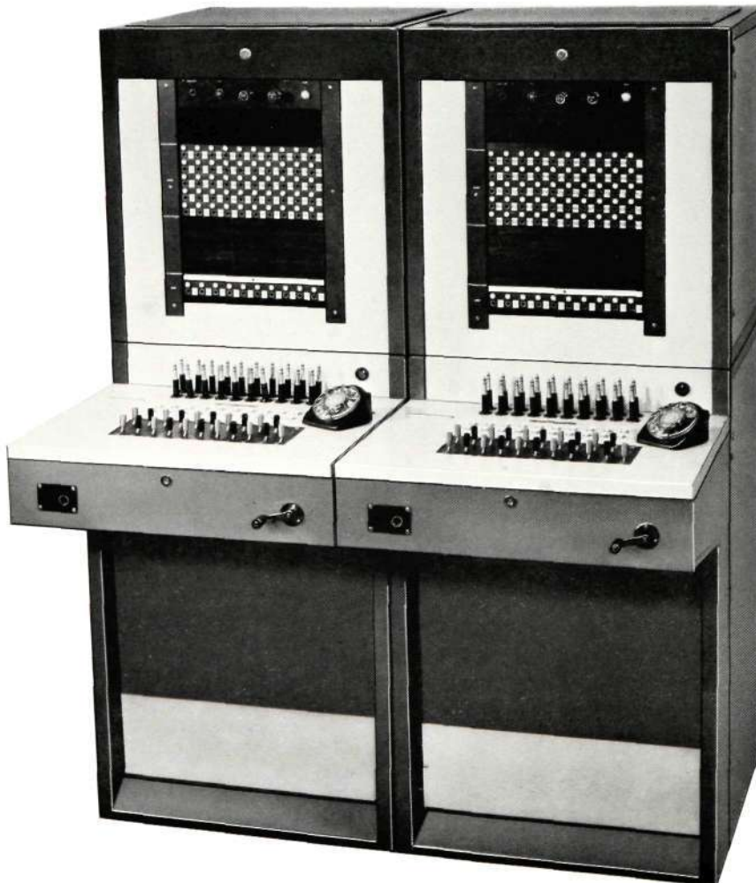
Figure 1— Fully assembled switchboards
