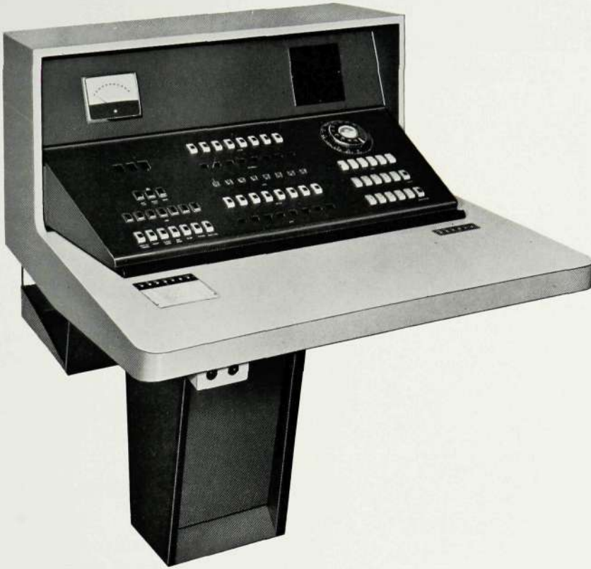
Figure 11—Pedestal-mounted console for PABX installation at the Plessey Company, Vicarage Lane, Ilford, Essex
