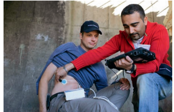
Lars Ruediger and Mehran Namazi test MobiMed telemedicine technology during the exercise. Patient data – in this case blood pressure and ECGs – is sent over the QuicLINK network to the field hospital.
