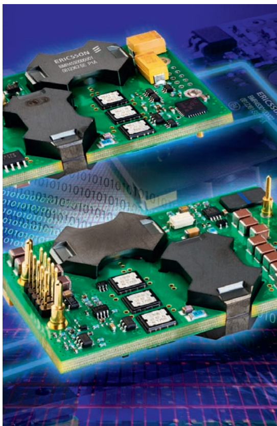
The two sides of the BMR453 power module, the digitally-controlled DC/DC converter, which is assembled onto a circuit board. The black components are transformers.
