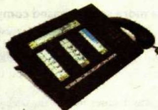
The Ericsson-developed broker telephone CTT11K can handle up to 250 connections at once.
