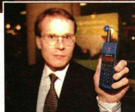
What seems to be a mobile telephone is actually something else. The TEMS Transmitter simulates a transmitting base station and is an important part of the system for simplified indoor planning of mobile networks, explains product developer Kari Korkala.
