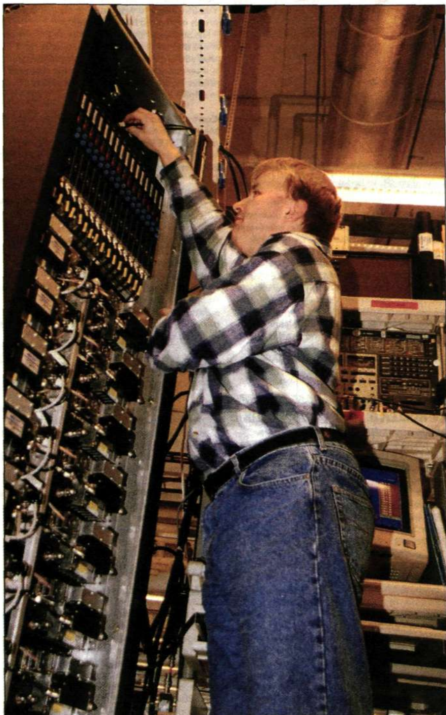
Claes Östlund applies final testing to an NMT base station that is to be delivered to an operator in Russia.
