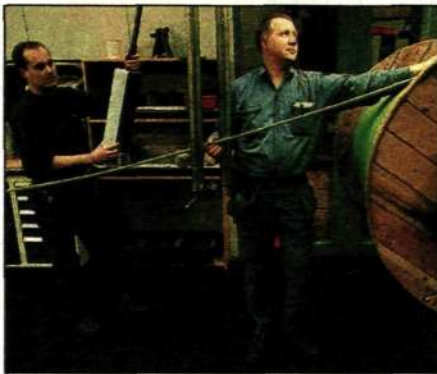
Per Flöjt and Jan-Erik Norin rolling up a fiber-optic cable that does not contain PVC but instead uses polyethylene with magnesium hydroxide as a fire retardant.
