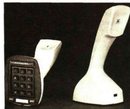
The Ericofon 700 was the world's first completely electronic one-piece push-button telephone
