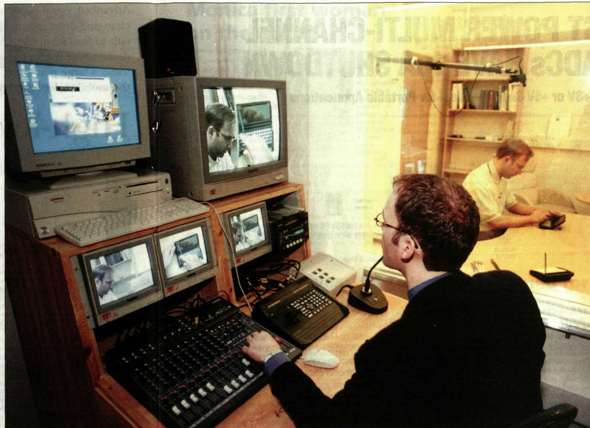
At the User Applications Lab in Kista, mobile telephone terminals and services are studied from the perspective of the end-user. All interfaces must be well thought out from a user-friendliness standpoint. Test subjects' work with the test products are closely studied with the help of cameras and microphones. And just as in a good spy movie, the analysis lab is hidden behind mirrored walls.
