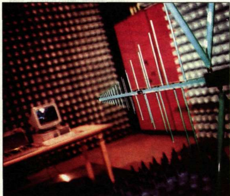
The Kumla plant has set up its own lab for measuring electromagnetic radiation and its effects. The lab is the most advanced of its kind in Sweden, says Savo Zabradac, who is in charge of the lab.
