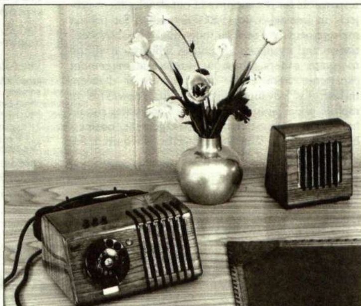
The DBF 1102 was one of Ericsson's first loudspeaker phones with freestanding loudspeaker. Both units were finished in walnut.
