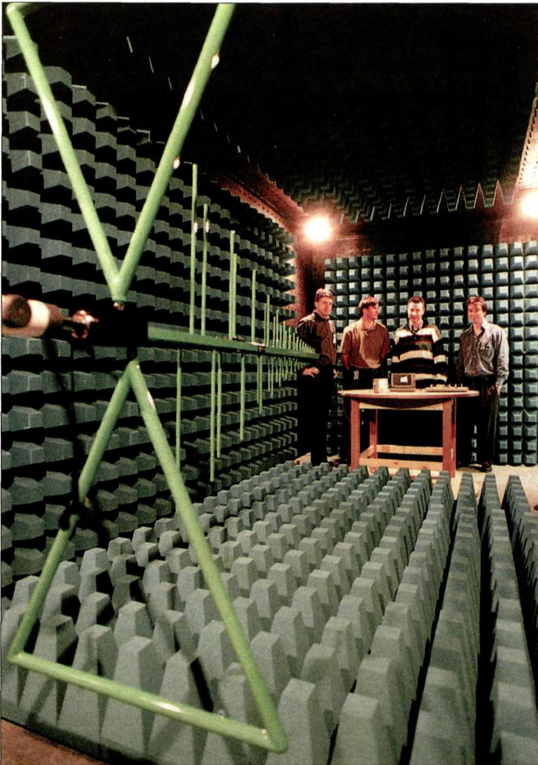
With a testing lab, it's possible to measure both how much electromagnetic radiation a mobile phone generates, and how much radiation it can withstand. The testing lab is designed to eliminate external interference.
