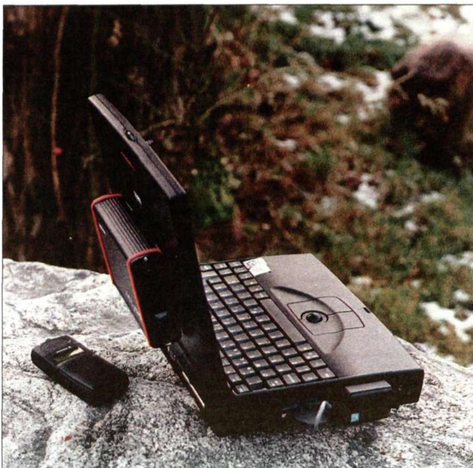
A DAB receiver, a laptop computer and a GSM telephone are being used to test the new AWIAN technology in Gothenburg. Users can download information from the Internet at speeds of up to one megabit per second.
