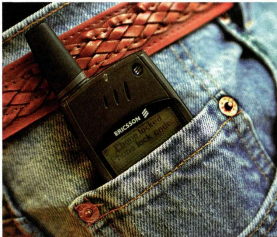
The T28 is the world's slimmest cellphone – just 15 millimeters thick – due largely to new battery technology, which Ericsson is the first to present, and the new 3-volt platform.
