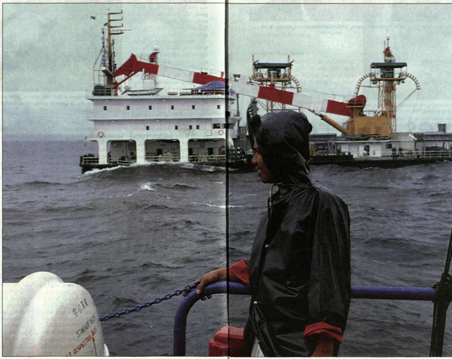
Networker, the specially built cable vessel, lays submarine cable 40 meters under the surface of the Gulf of Thailand. A large steel sword is positioned against the seabed and, supported by a water injector, digs a trench 1.5 meters deep into the ocean floor. The work is monitored by divers, who also carry out precision work when the cable crosses encountered, for example. During installation, the cable is connected to test equipment
