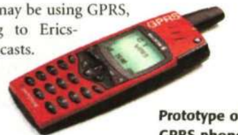
Ericsson showed a complete GPRS system at CeBIT, where users could try various mobile data services using a prototype GPRS phone based on the R320.
