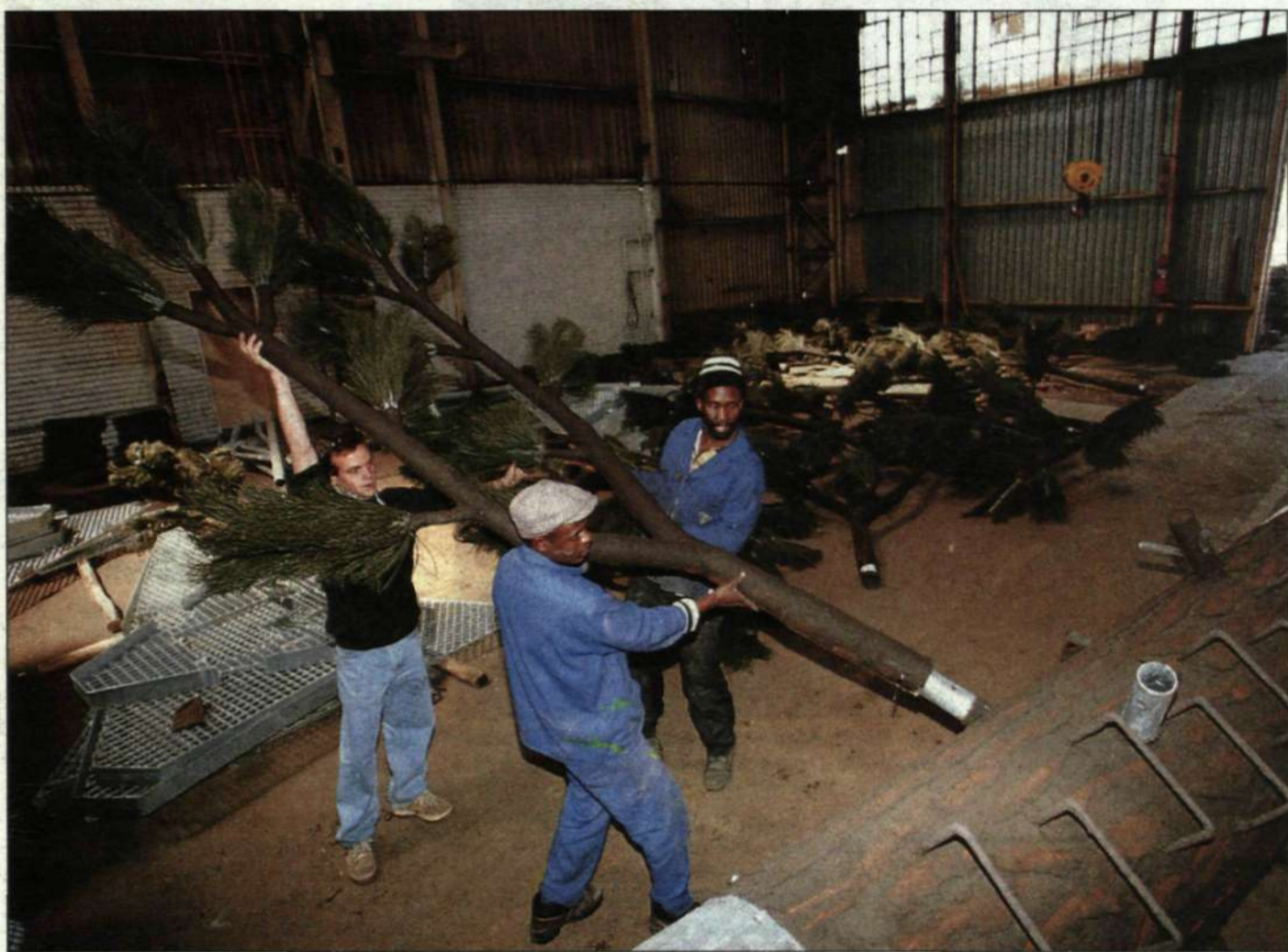
Lawrence Ambrose, Lucas Selepe and David Zapeei assemble branches on the "trees" used to camouflage radio masts in South Africa.
