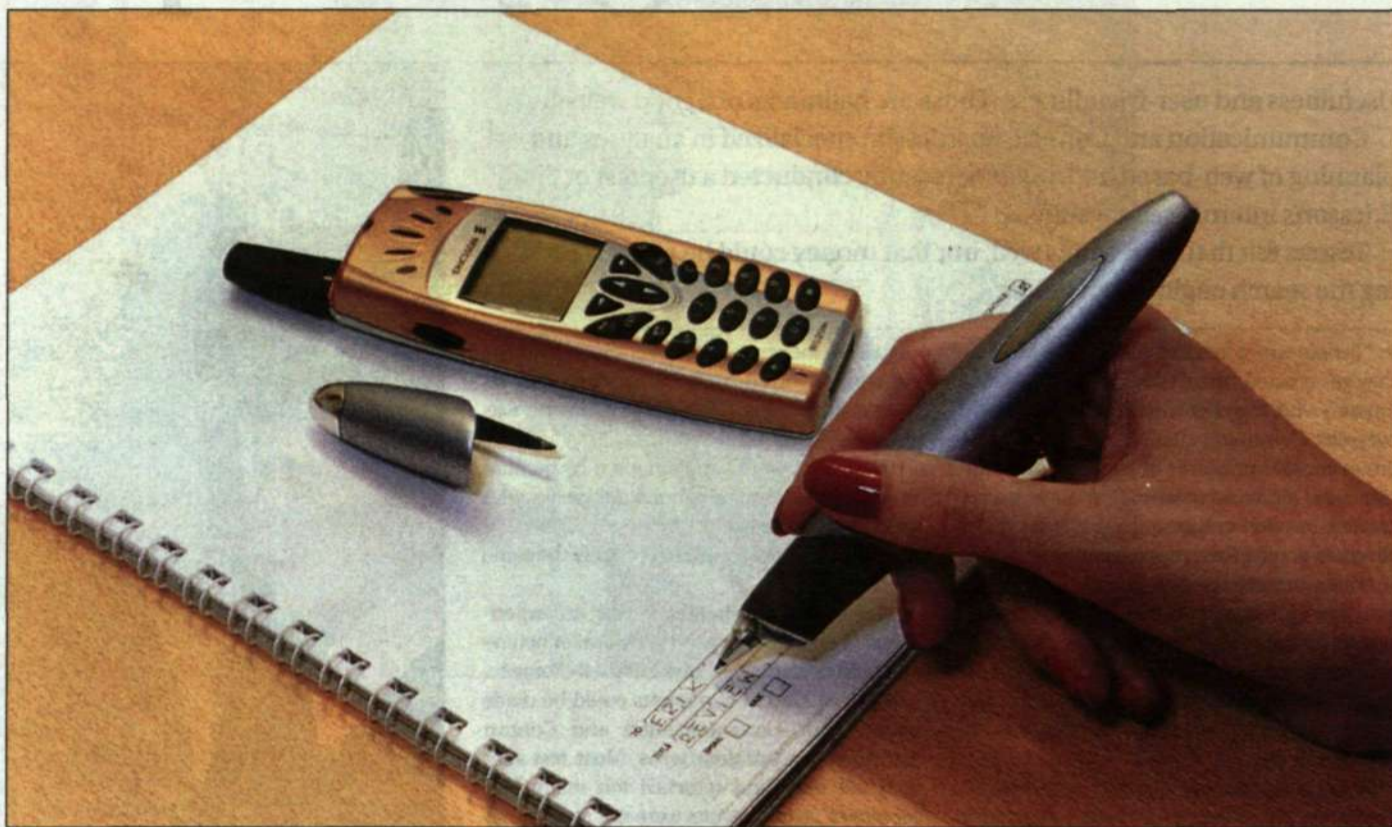
Using a Chatpen on special paper eliminates the need to input text by way of a phone keypad or computer keyboard. Both e-mails and faxes can be sent directly from a sheet of note paper that has been printed with Anoto's dot pattern.
