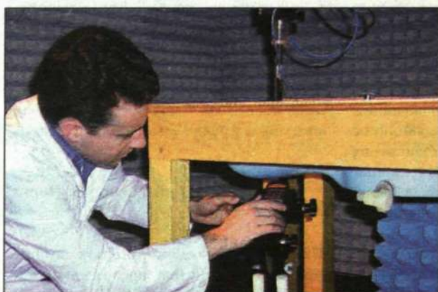
Electromagnetic fields are measured at the Ericsson EMF research laboratory in Kista. Research Engineer Martin Siegbahn places a mobile phone in a holder behind a plastic shell filled with a liquid with the same electrical properties as the tissue in the human head.
