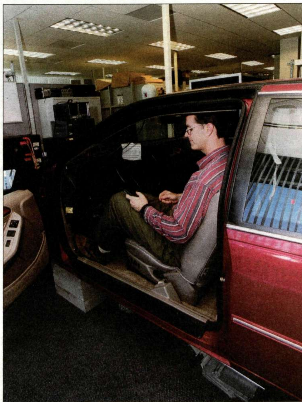
Speech audibility testing against a background of vehicle and traffic noise recorded in urban environments all over the world. Michael D. Townsend is at the controls.
