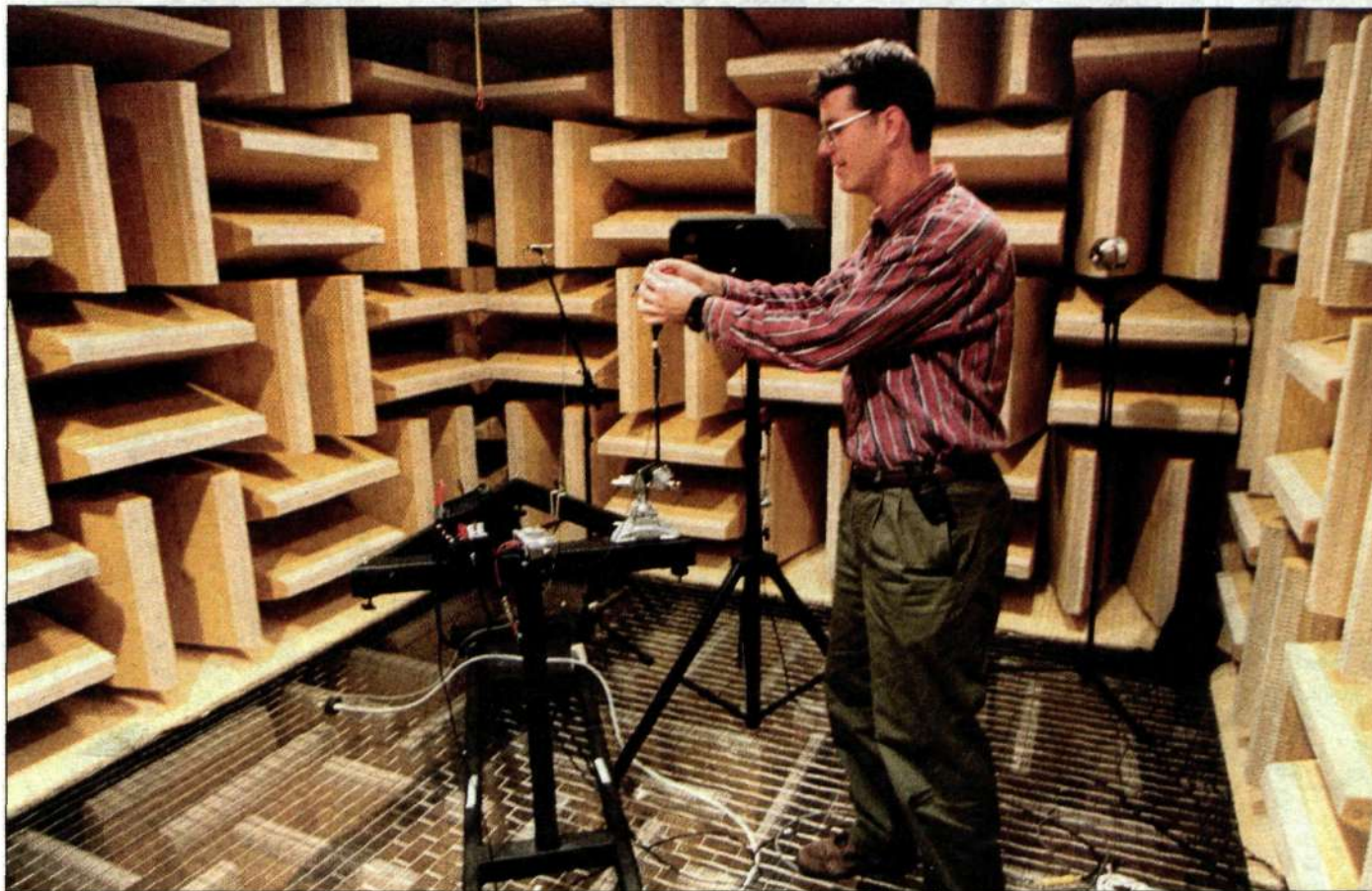
In this room, measurements are taken to see how well various sounds are picked up by mobile phones. This is one of many tests that Ericsson phones are subjected to in the test laboratory at Research Triangle Park in the US. Michael D. Townsend, a sound engineer at the lab, explains how virtually all sound waves are absorbed by the cone-shaped protrusions lining the walls. Photo: Ecke Küller
