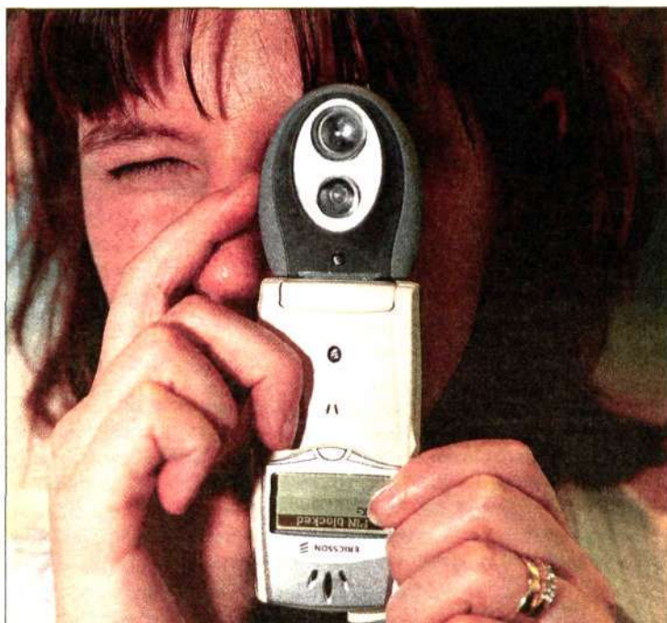
Camera instructions are listed on the telephone display and selections are made using the keypad. Photo: Ecke Küller
