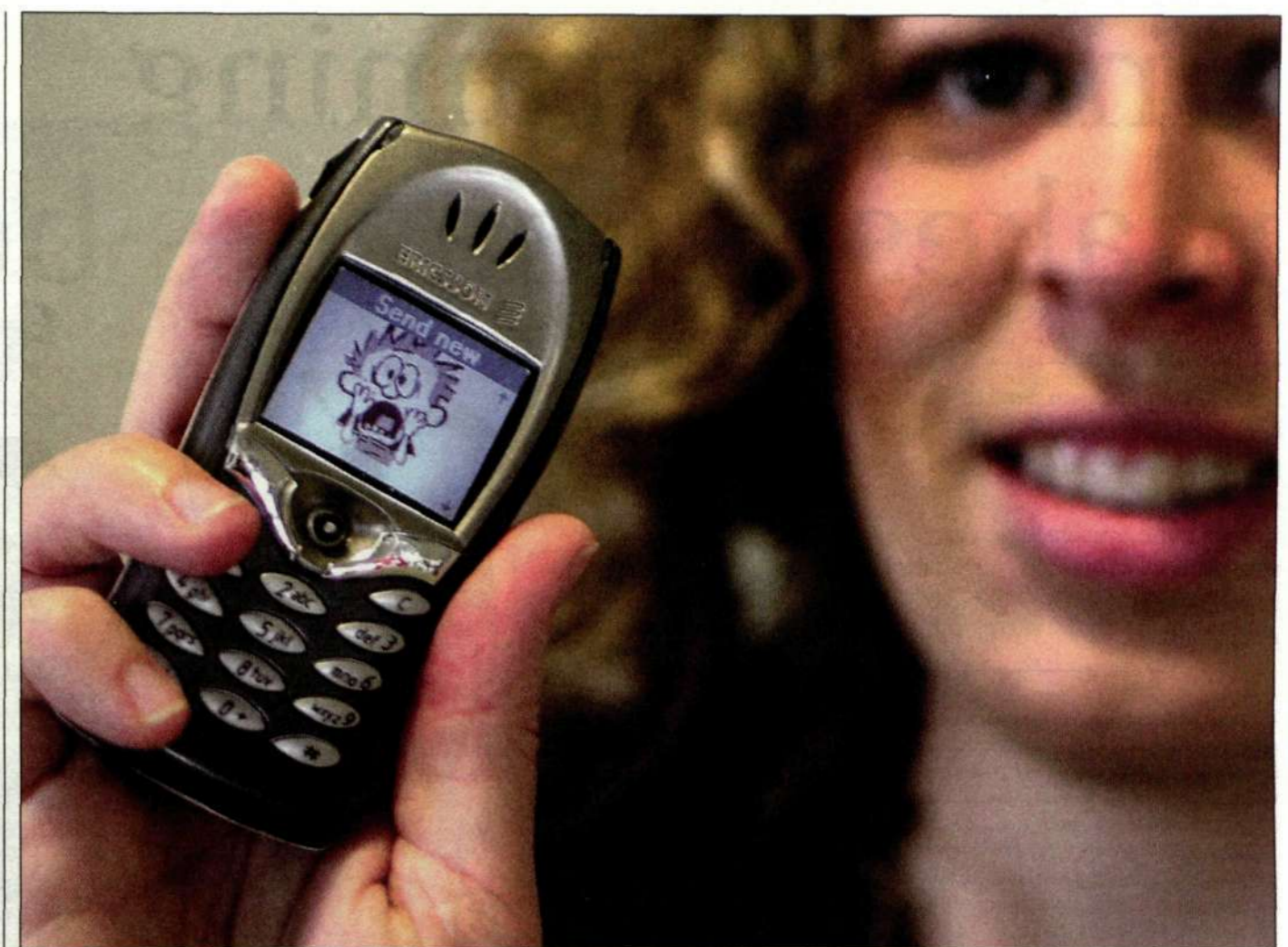
MMS, Multimedia Messaging Service, is an enhancement of the popular SMS service in which users can send short text messages between mobile phones. With MMS, it will also be possible to send moving images, digital sound, melodies and text.
