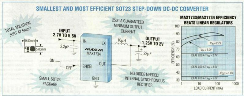
The MAX1733/MAX1734 feature a proprietary current-limited control scheme that operates at up to 1.2MHz, permitting operation with physically small external components.
