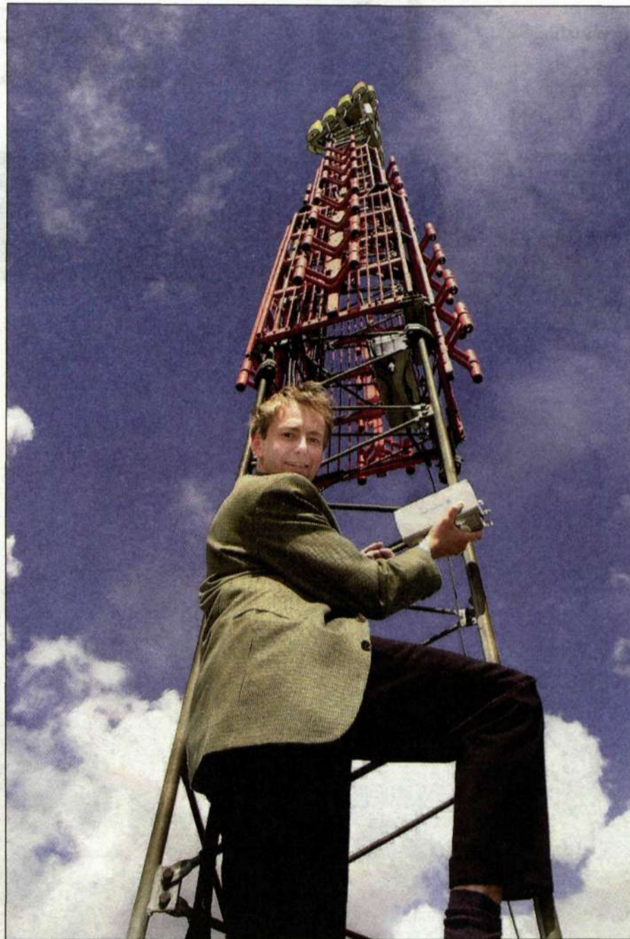
Ulf Sundström demonstrates the TMA amplifier, which is mounted on the mast near the antenna where it boosts signals received from mobiles.
