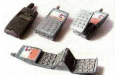
With a fold-out keyboard on the Cool Tool it will be easier to send e-mails from the phone.
