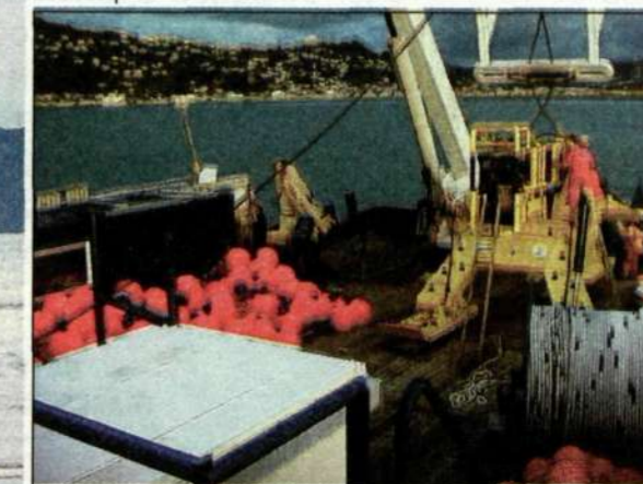
After a 52-day voyage across the world's oceans, Searanger arrives in Christchurch, New Zealand. The ship's cargo included buoys, 349 kilometers of sea cable and a plough for burying the cable.
