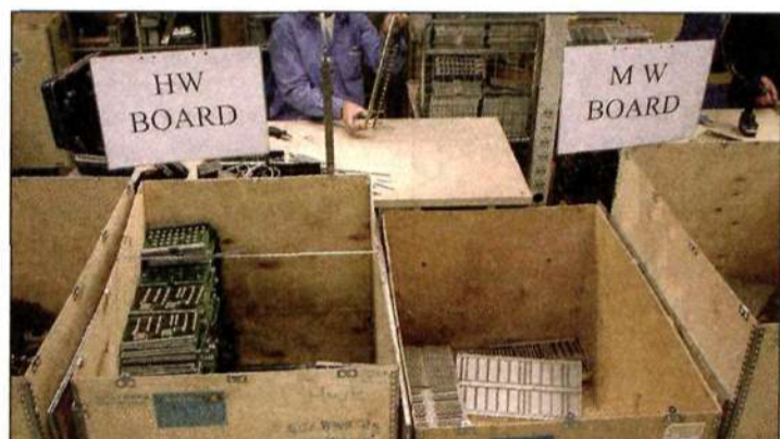
Ericsson ships the dismantled material to special collection centers, such as this site in Rijen, in the Netherlands. The material is separated by source before it is sent to subcontractors for recycling.
