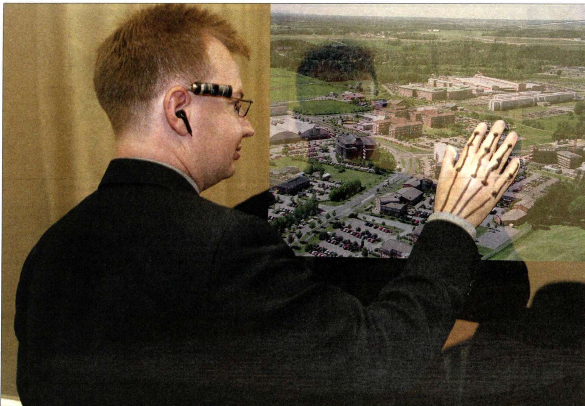
Using all of our senses opens new opportunities for integrating people and technology. Martin Rantzer demonstrates a future scenario where a projector on the side of his glasses projects a virtual image onto the lens. Together with a glove with built-in sensors and force-feedback, which provides a sense of touch, he can see and feel a three-dimensional image, which does not exist.
